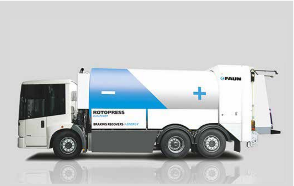
The first waste collection vehicles with diesel-electric hybrid drive developed by Faun Zoeller (UK).
